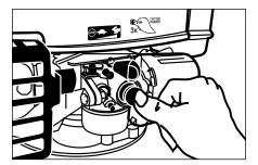
**Step 6** Push primer ball three times. Wait 3 seconds between each push.
