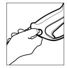
**Step 6** Disconnect the high pressure hose from the high pressure outlet and engage the gun safety lock.
