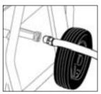
**Step 5** Disconnect the garden hose from the water inlet on the unit.
