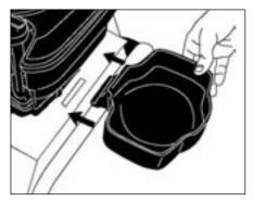
**Step 4** Insert the detergent tray into the tray slot and screw in the fastener. Fill the detergent container with the proper detergent for you cleaning project. Note: Place the container on the tray.
