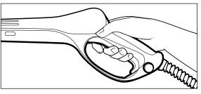
**Step 4** Trigger the gun to eliminate trapped air, wait for a steady flow of water to emerge from the spray nozzle.
