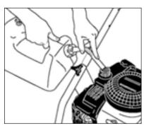
**Step 5** Fill gas tank with unleaded gasoline. Do not use leaded gasoline.
