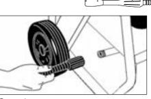
**Step 1** Connect the high pressure hose to the unit's high pressure outlet.
