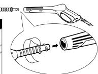
**Step 2** Insert the Vario spray wand into the gun. Push in and turn clockwise to lock spray wand in place.
