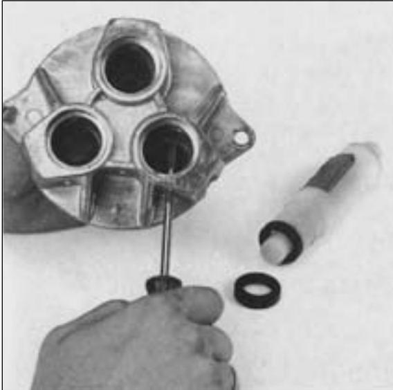
Remove the housing together with the pistons.
