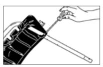
**Step 2** Align the holes of the accessory rack to the handle and fasten the four (4) screws.
