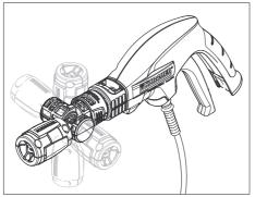
**Note:** The adjustability of the spray lance head ensures easier access to hard-to-reach places.
