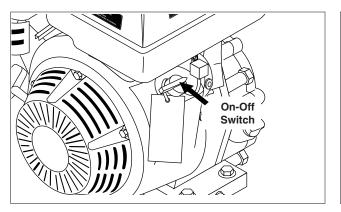
**STEP 8:** Turn the engine switch to "On" position. On Vanguard engines, move the throttle lever to "Fast" position, shown on the engine as a rabbit.
