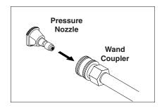
**STEP 6:** Pull spring-loaded collar of the wand coupler back to insert your choice of pressure nozzle.
