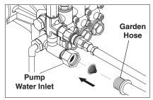
STEP 10: Check inlets filters, remove debris, then connect the garden hose to pump water inlet. CAUTION: Do not run the pump without water or pump damage will result.
