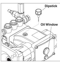
**STEP 2:** Remove shipping cap and install oil dipstick. Check pump oil level by using dipstick or observe oil level in oil window (if equipped). Use 40 wt. non detergent oil.
