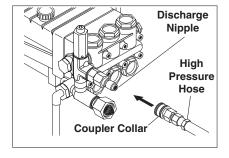
**STEP 9:** Connect the high pressure hose to the discharge nipple. Push coupler collar forward until secure.
