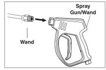
**STEP 6:** Attach wand to spray gun. Tighten wand.
