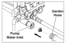
STEP 11: Check inlets filters, remove debris, then connect the garden hose to pump water inlet. CAUTION: Do not run the pump without water or pump damage will result.
