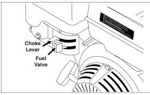
**STEP 7:** Move the choke lever to the "Choke" position (on a warm engine, leave the choke lever in the run position). Move the choke lever to the "Closed" position. To restart a warm engine, leave the choke lever in the "Open" position.
