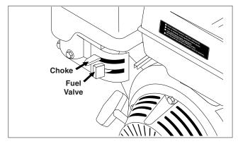
**STEP 6:** Rotate the fuel shut-off valve to the "On" position. Slide the fuel valve lever to the "ON" position. When the engine is not in use, leave the fuel valve in the "OFF" position.
