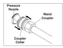
**STEP 8:** Release the coupler collar and push the nozzle until the collar clicks. Pull the nozzle to make sure it is seated properly.
