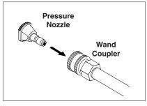
**STEP 7:** Pull spring-loaded collar of the wand coupler back to insert your choice of pressure nozzle.
