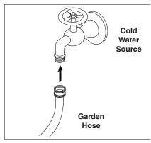
**STEP 4:** Connect garden hose to the cold water source and turn water on completely. Never use hot water.
