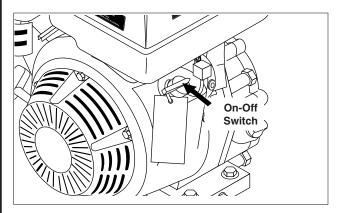
**STEP 8:** Turn the engine switch to "On" position. On Briggs engines, move the throttle lever to "Fast" position, shown on the engine as a rabbit.
