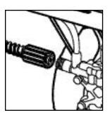
Step 6 Connect the high pressure hose to the unit's high pressure outlet.
