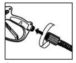
Step 5 Attach the high pressure hose to the spray gun.
