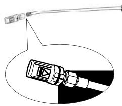
Step 1 Use triple jet nozzel (set to CHEM. position) to apply detergents
