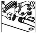
Step 5 Disconnect the garden hose from the water inlet on the unit.
