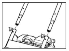
Step 1 Attach the handle to the frame of the pressure washer. Align holes, insert bolts, and tighten with knobs.
