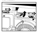
Step 5 (Briggs & Stratton) Turn fuel valve to "ON". Slide the throttle control to the fast position. Move the choke lever to the "CHOKE" position (only if the engine is cool). After starting, move the choke to "RUN".
