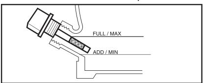
Be sure the machine is level when checking the oil level. (Refer to the engines operating manual for seasonal grades).
