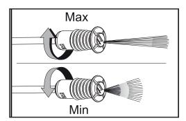
→ For lower pressure turn the wand collar in the minus (Min) direction.
