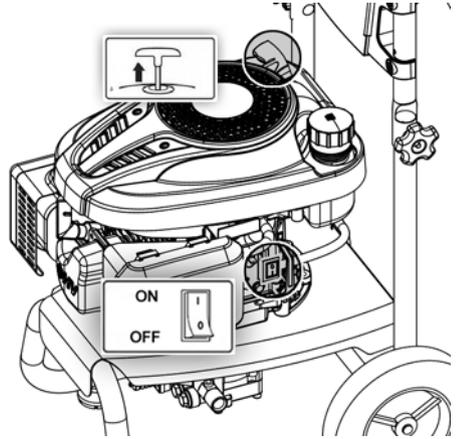
1. Turn the engine switch to "ON" position.
