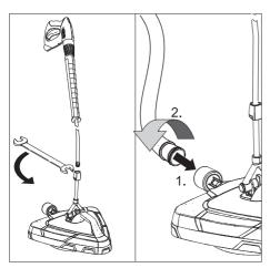
→ Connect the steel pipe of the high pressure cleaner to the surface cleaner and tighten it with a wrench (opening width 24).
