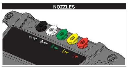
The five color-coded quick connect nozzles provide a wide array of spray widths from  $0^{\circ}$  to  $40^{\circ}$  and are easily accessible when placed in the convenient rubber nozzle holder, which is provided on the front of the machine.
