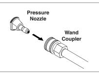
**STEP 8:** Pull spring-loaded collar of the wand coupler back to insert your choice of pressure nozzle.
