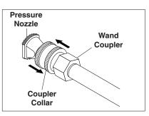
**STEP 9:** Release the coupler collar and push the nozzle until the collar clicks. Pull the nozzle to make sure it is seated properly.
