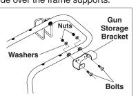
**STEP 4:** Attach the gun storage bracket and insert bolts from the outside, place washers through bolts from inside and insert nuts from inside as well. Tighten nuts.
