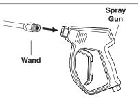
**STEP 7:** Attach wand to spray gun/ wand. Tighten both.
