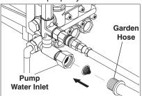
STEP 12: Check inlets filters, remove debris, then connect the garden hose to pump water inlet. *CAUTION: Do not run the pump without water or pump damage will result.*
