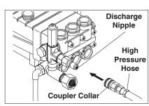
**STEP 10:** Connect the high pressure hose to the discharge nipple. Push coupler collar forward until secure.
