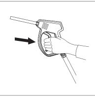
**STEP 5:** Trigger the spray gun to eliminate trapped air then wait for a steady flow of water to emerge from the spray nozzle.
