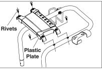
**STEP 5:** Attach the plastic plate from the top aligned to the four holes placed on top of the handle and insert the rivets through holes of plastic plate.
