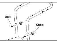
**STEP 2:** Insert the carriage bolt through the holes from the front of the unit and attach a knob from the back of the machine. Tighten Knobs with your hands.
