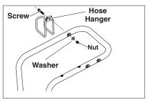
**STEP 3:** Attach the hose hanger and insert screw from outside, place washer through screw from inside and insert nut from inside as well. Tighten nut.
