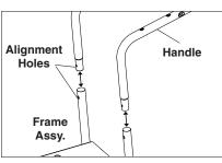
**STEP 1:** Attach the handle to the frame of the pressure washer. **Note**: It may be necessary to move the handle supports from side to side in order to align the handle so it will slide over the frame supports.
