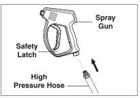
**STEP 6:** Attach the high pressure hose to the spray gun using teflon tape on hose threads.
