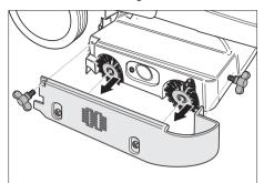
Remove both roller brushes, insert new ones (note hexagon fixtures for the roller brushes).
