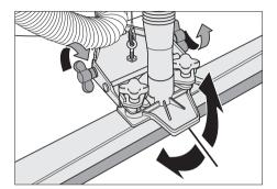
■ Tighten the wing nuts.
