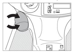
Adjust the brush contact pressure with the star knob.
