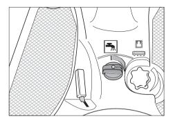
Control the water flow rate by depressing the metering pedal. Simultaneous depression of the drive and metering pedals ensures that metering is speed-dependent.
