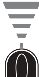
Low pressure fan jet for detergent injection
