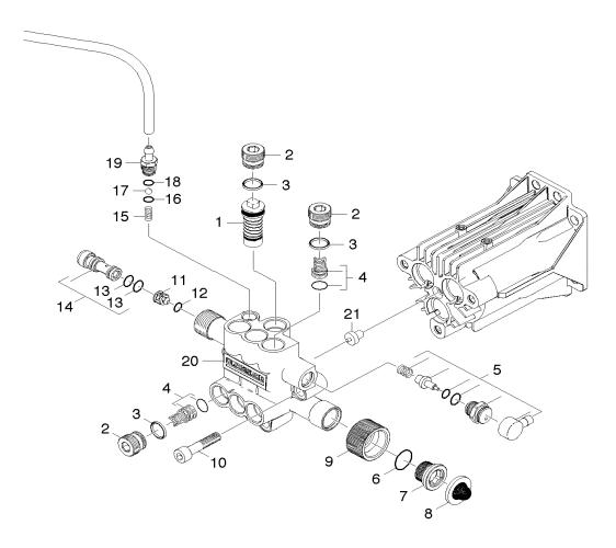
Part # 1 makes up Part # 9175-0070 Spill (Unloader) Valve
