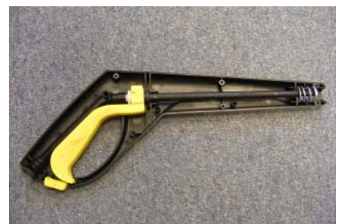
Place small spring inside inlet tube, 45 degree angle end then place inside white bushing end with single o-ring. Reassemble outer housing.
