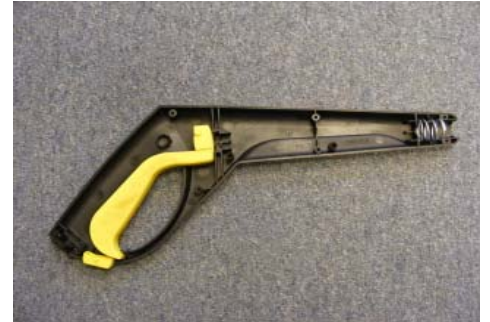
Insert trigger handle into housing
