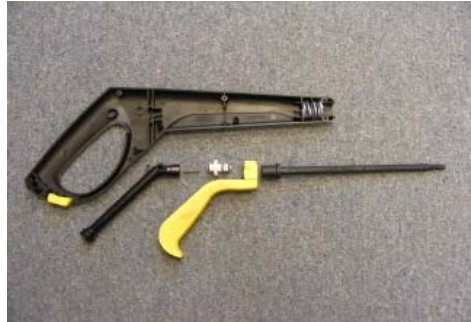
Insert large spring inside grooves at end of barrel
