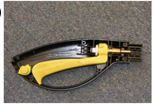
Insert plastic bushing through trigger handle into brass nozzle
