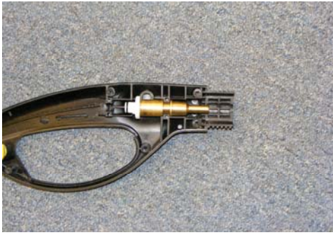
Shows placement of brass nozzle & plastic bushing
