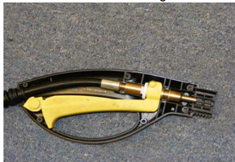
Final inside view of assembly.
