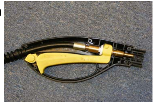
Insert spring into hose tip then insert hose tip into plastic bushing
