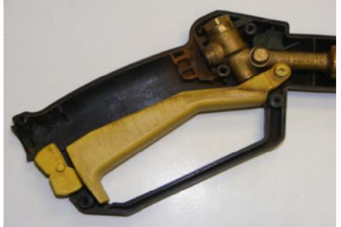
Install & placement of trigger lock.
