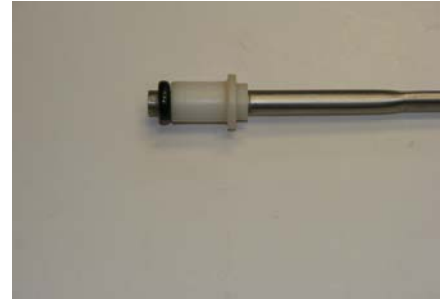
Slide white plastic sleeve onto metal pipe, place o-ring onto end of pipe.
