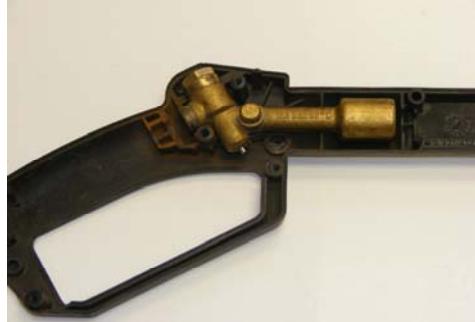
Placement of brass manifold inside trigger gun housing
