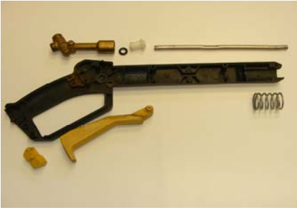
Internal parts of Trigger Gun 4775-2640 Version 1 (older style)
