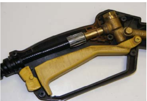
Install & placement of high pressure hose.
