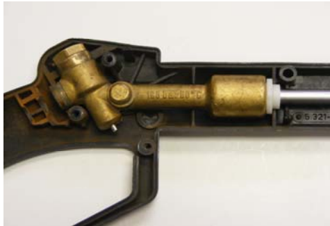
Placement of picture 4 components in trigger gun housing.
