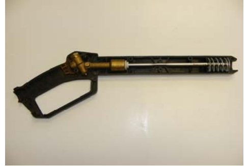
Install & placement of spring at end of barrel of trigger gun.
