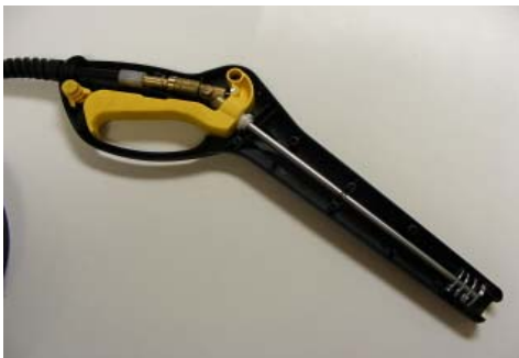
Final inside view of assembly with hose
