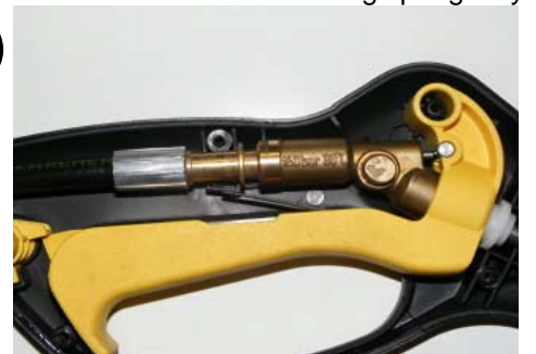
Close-up view of final assembly with hose
