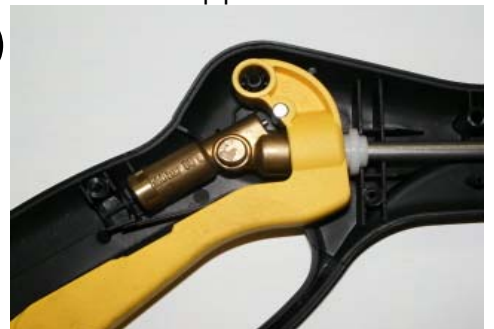
Insert o-ring, plastic sleeve & pipe through trigger handle into brass manifold
