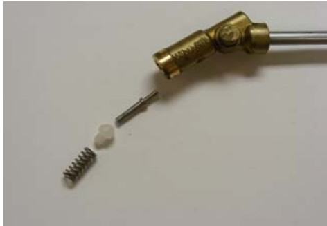
Plunger bar, valve disc & spring in order of insert into brass manifold
