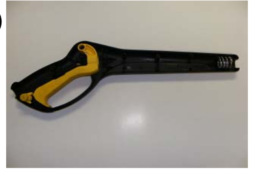
Place large spring in grooved area on barrel & place trigger handle into housing
