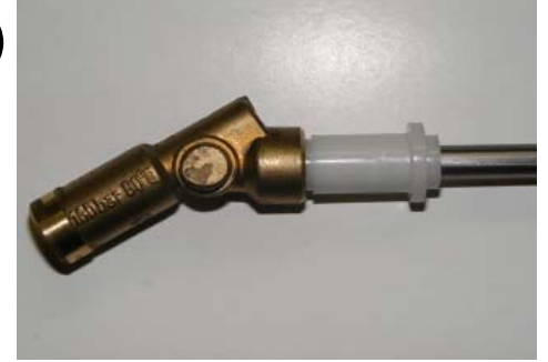
How manifold, o-ring, plastic sleeve & pipe looked assembled.
