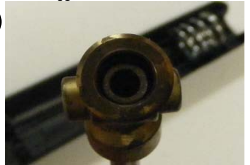
Looking into bottom of brass manifold showing spring only
