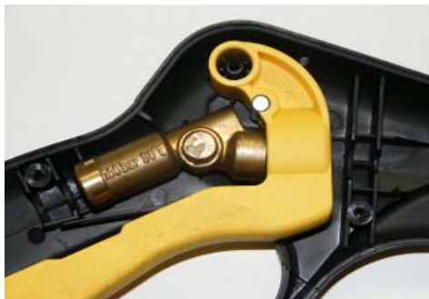
Insert brass manifold through trigger handle
